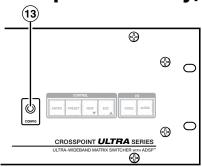
Figure 2-24 — Front panel configuration port
